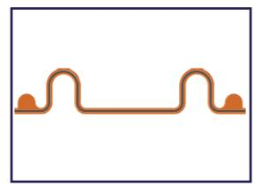
Beaded Flange Crimped Diaphragm
